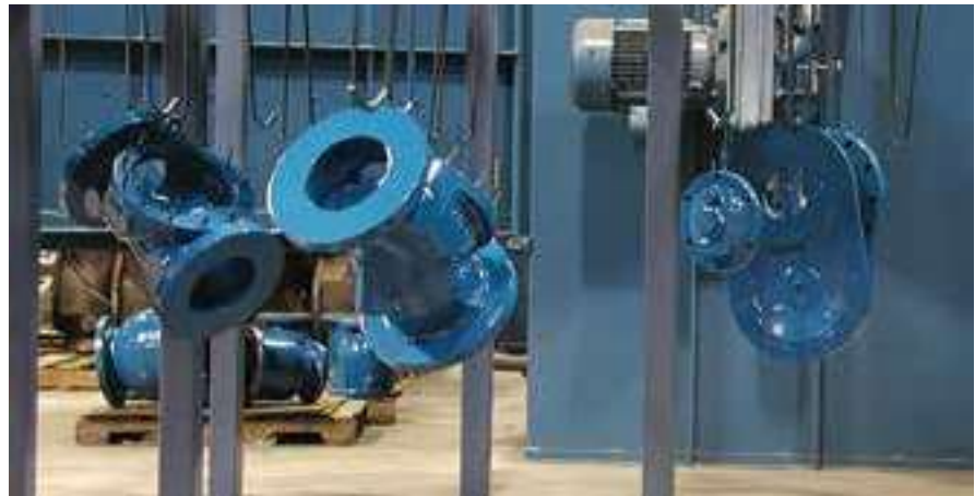
Figure 1 – Fusion bonded epoxy coating on valve castings.
