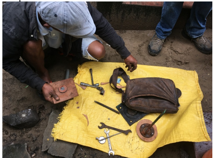
Pump manufacturer Nary making an adaptation of piston valve with Fe components.
