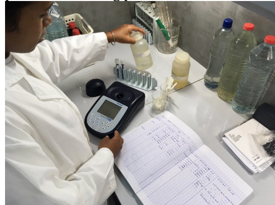
Setting up for testing physico-chemical parameters using photometer.
