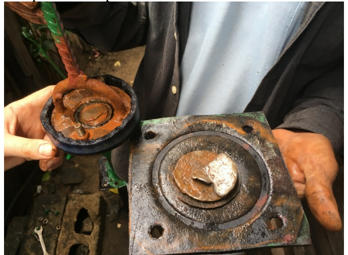
A pump before adaptation showing lead components in piston and foot valves.
