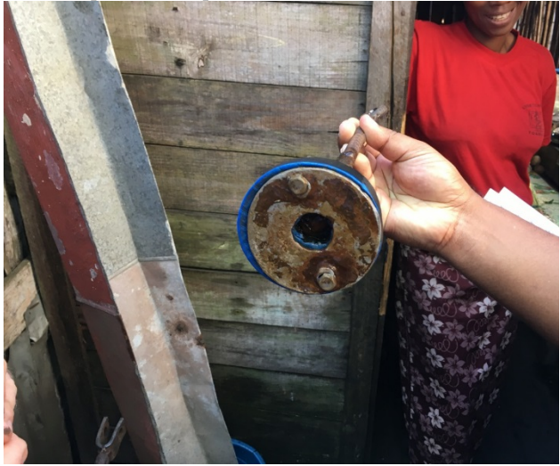
Close-up view of piston valve.
