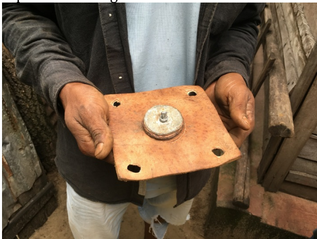
New foot valve parts: The two check valves consists of leather and an iron weight to replace lead weight.
