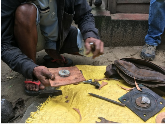
Second photo of pump manufacturer Nary making an adaptation of valve with Fe components.
